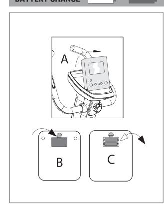
A weak or an extinguished computer display makes a battery change necessary. The computer is equipped with two batteries. Perform the battery change as described below:
